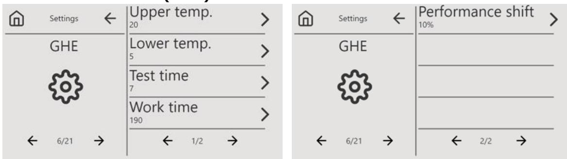
Fig. 27 Screens of ground heat exchanger setting parameters
