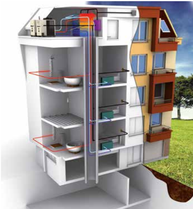
Application in summer and winter operation with underfloor heating system, fan coils
