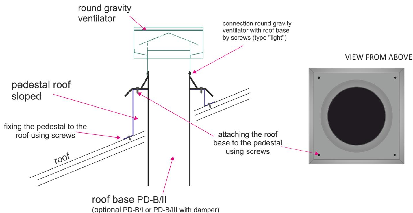
**W2** - Installation visible with mounting flanges (EXAMPLE) - recommended at the elements above f 400.
