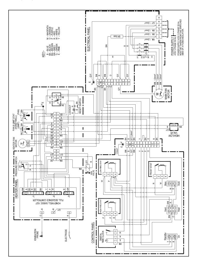
Wiring Diagram 33-66-210 PV250-490 HI/LO CP2 Controls 415/50/3ph
