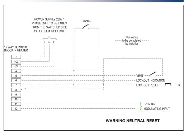
Less Controls Connections Modulation 1 Phase 33-64-584
