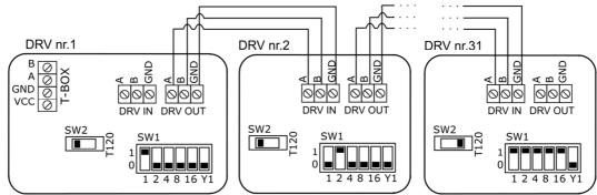
• In last DRV in line, DIP-switch SW2 has to be switched to the right -T120W
