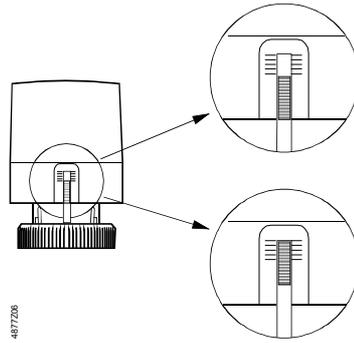
In this position, the actuator is de-energized:
