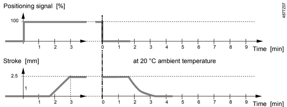
The positioning time depends on the voltage and the ambient temperature.
