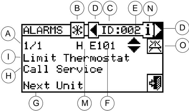
The screenshot shows the Alerts Menu interface. At the top, it says 'ALARMS' followed by a plant icon and a scroll bar. Below that, it displays 'ID:002' and a unit icon. The main area shows '1/1 H E101' with a scroll bar, 'Limit Thermostat', 'Call Service', and 'Next Unit' with a scroll bar. Callout letters A through O are placed around the screen to identify specific features.
