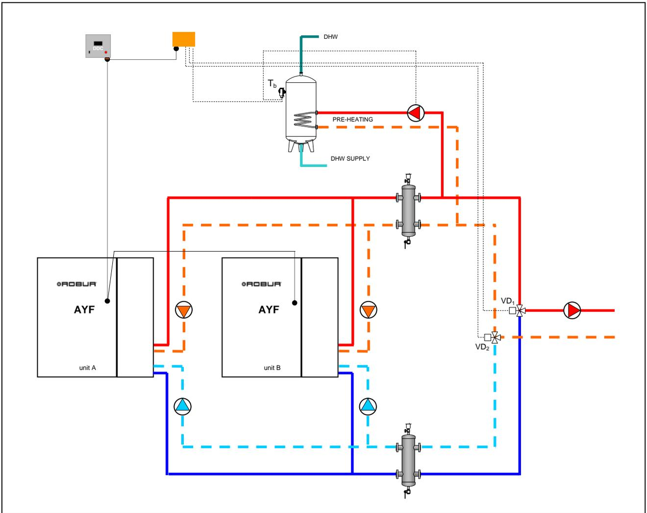
**Figure 24 - SE OF DHW IN COOLING MODE**
