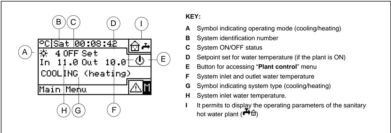
**Figure 25** – EXAMPLE OF INITIAL SCREEN FOR CONTROLLING TWO-LINE COOLING/HEATING PLANTS
