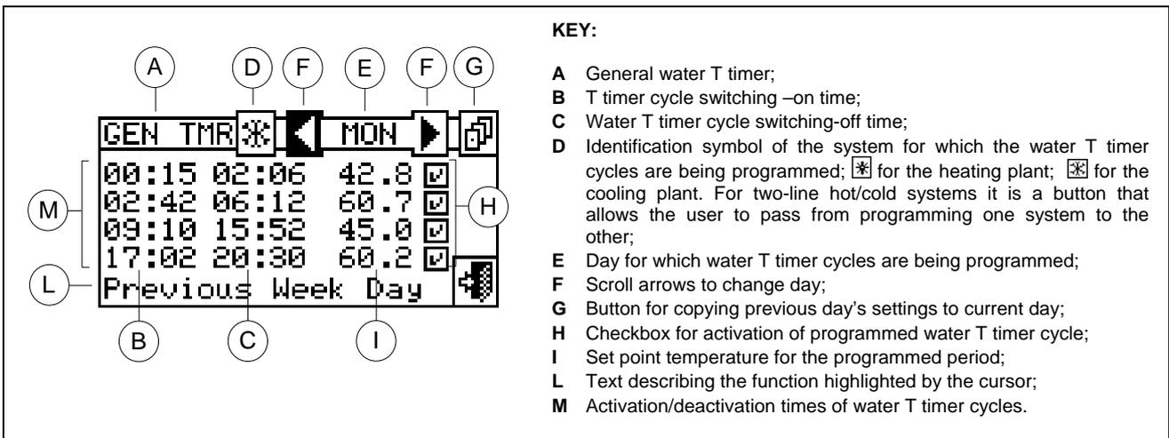
**Figure 7 – PROGRAMMING SCREEN FOR GENERAL WATER T TIMER CYCLES**
