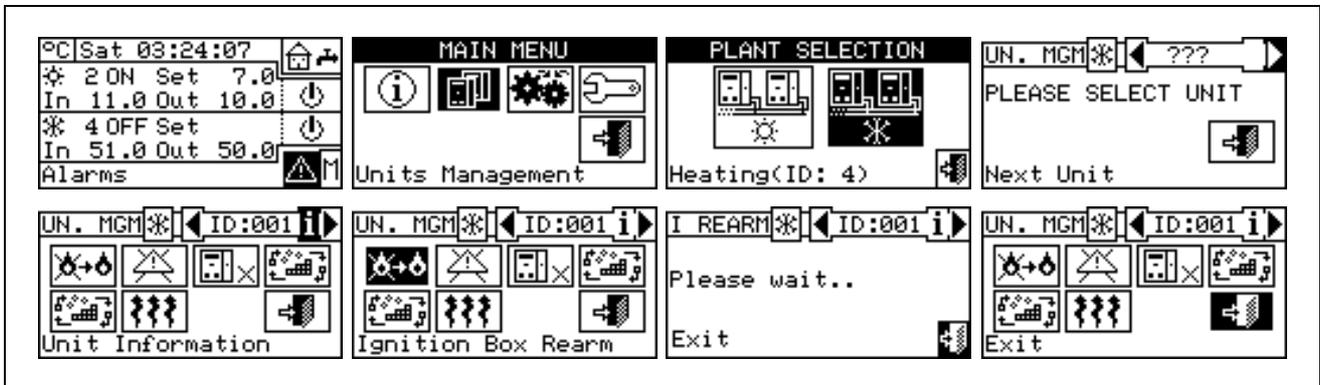
The flame control unit can be reset also by accessing the "Errors" menu
