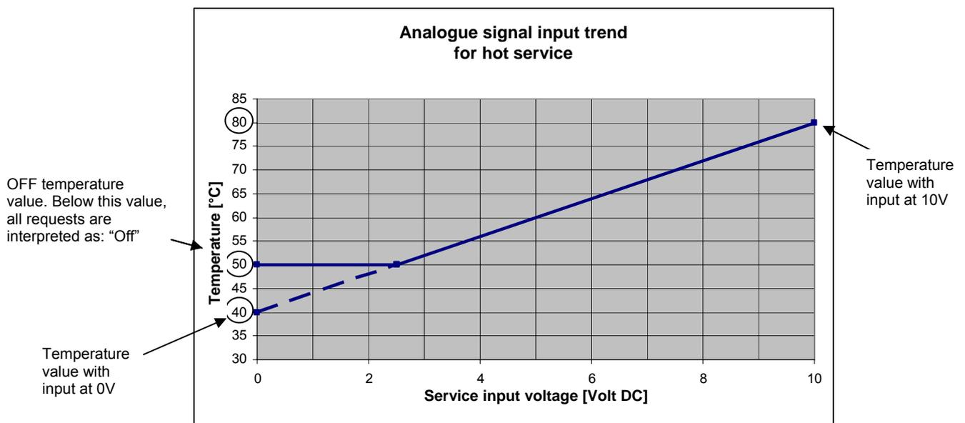
**Figure 3** Voltage signal input trend for hot analogue service (heating, DHW0 and DHW1)
