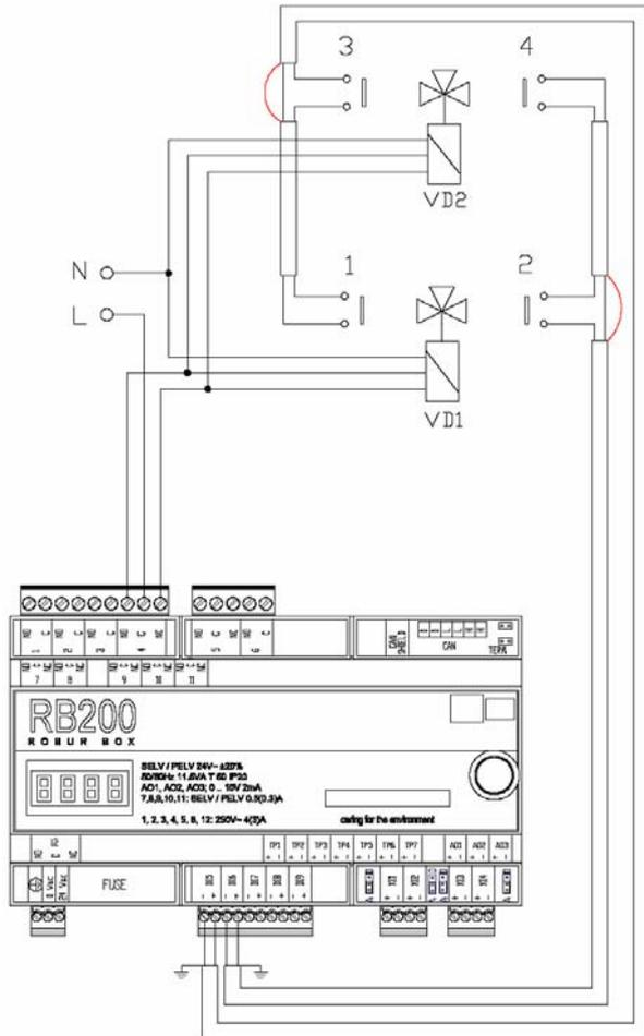
Example of connection with limit switch auxiliary contacts open in the limit switch position
