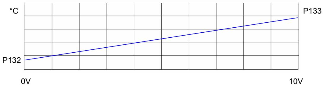
**Figure 5** Correspondence between generator service temperature and voltage
