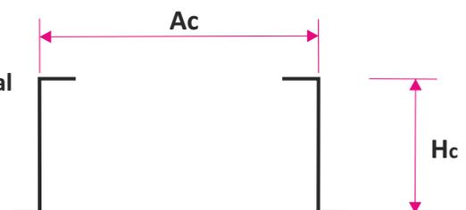
The height of the straight and angle pedestal adjusted to the conditions at its mounting location (need to define at the time of making order).
