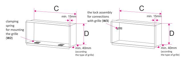
Attaching the frame to the wall with mounting hole
