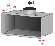
SR-Gw - plenum box with the spigot on the top
