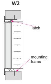
Assembling invisible by latches in grille and mounting frame RM or in plenum box.
