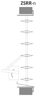
The shutter is adjusted manually using a common guide located behind the blades
